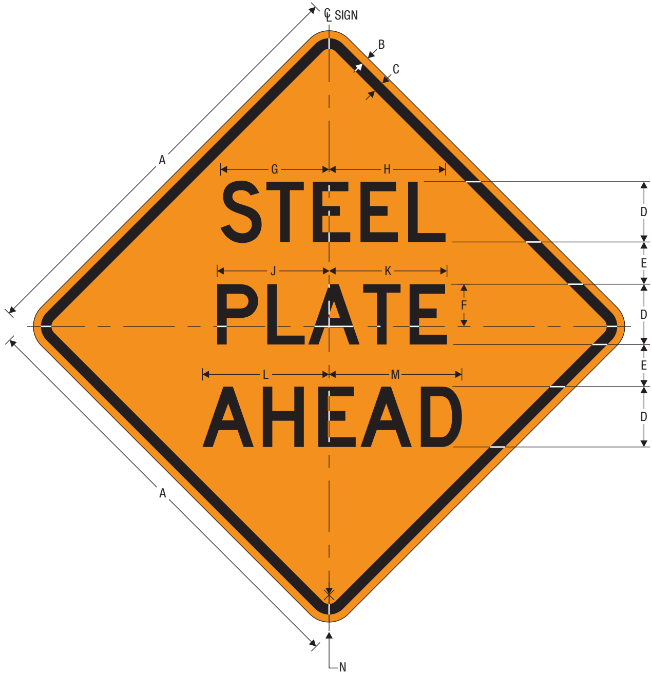
W8-24 STEEL PLATE AHEAD
