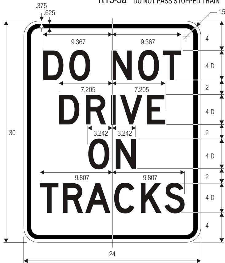
R15-6a DO NOT DRIVE ON TRACKS
