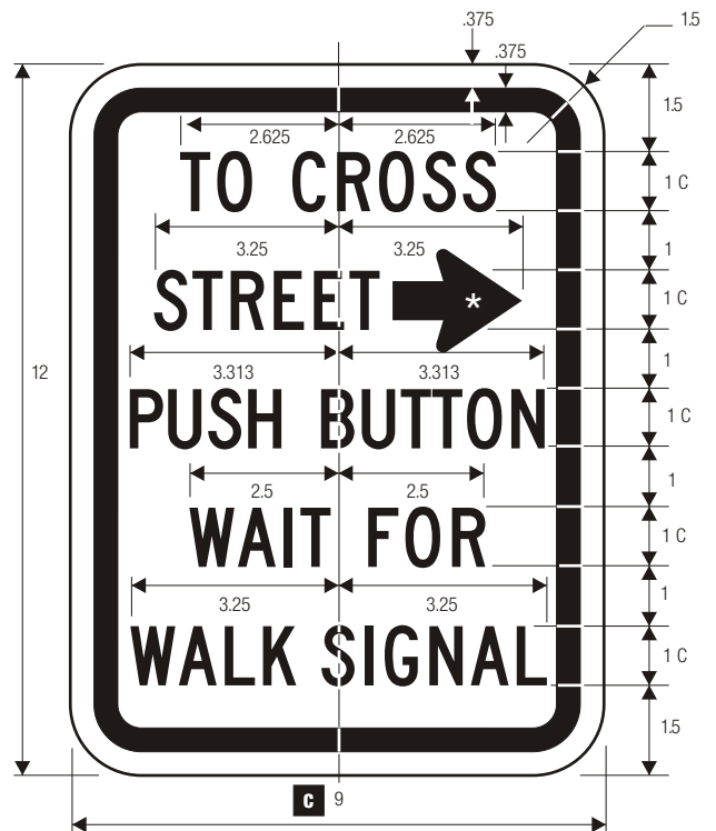
R10-4a PEDESTRIAN TRAFFIC SIGNAL
