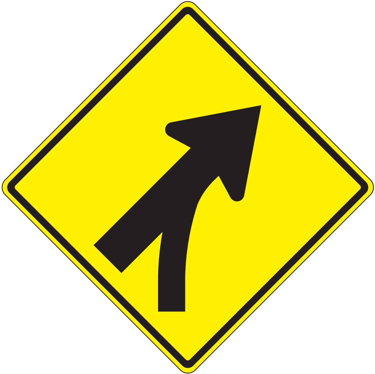
W4-5R Entering Roadway Merge (right)
