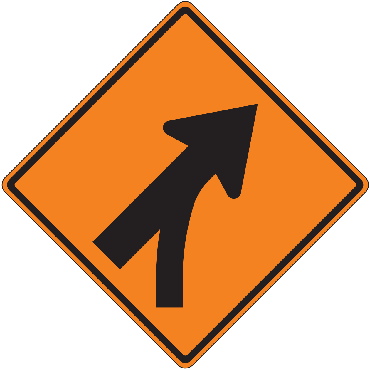
W4-5R Entering Roadway Merge (right)
