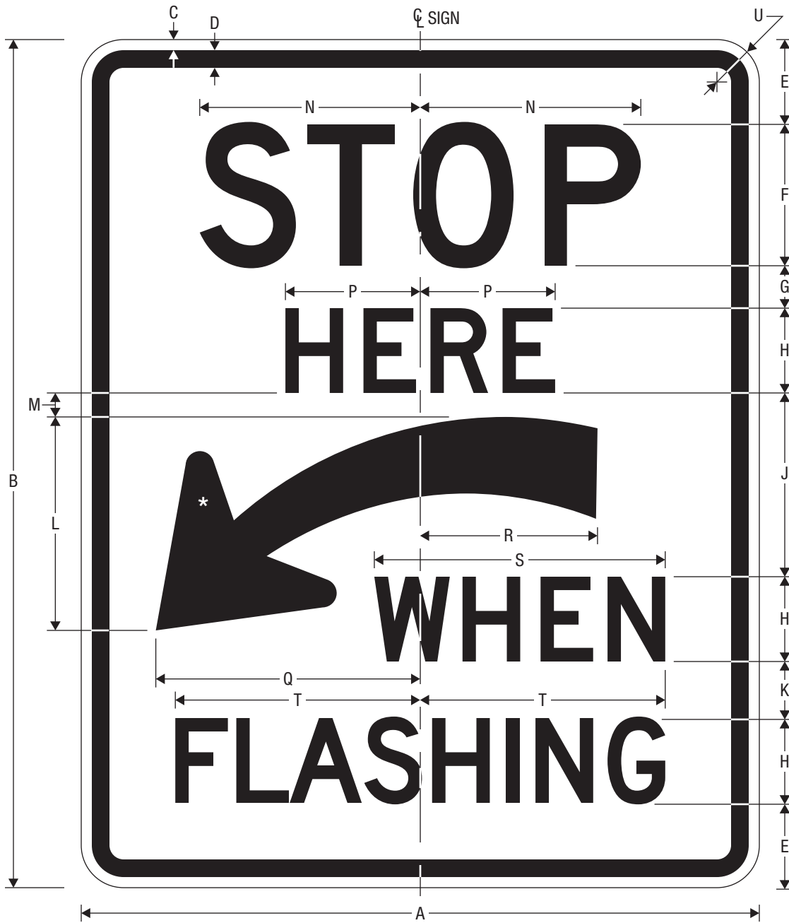
R8-10a STOP HERE WHEN FLASHING
