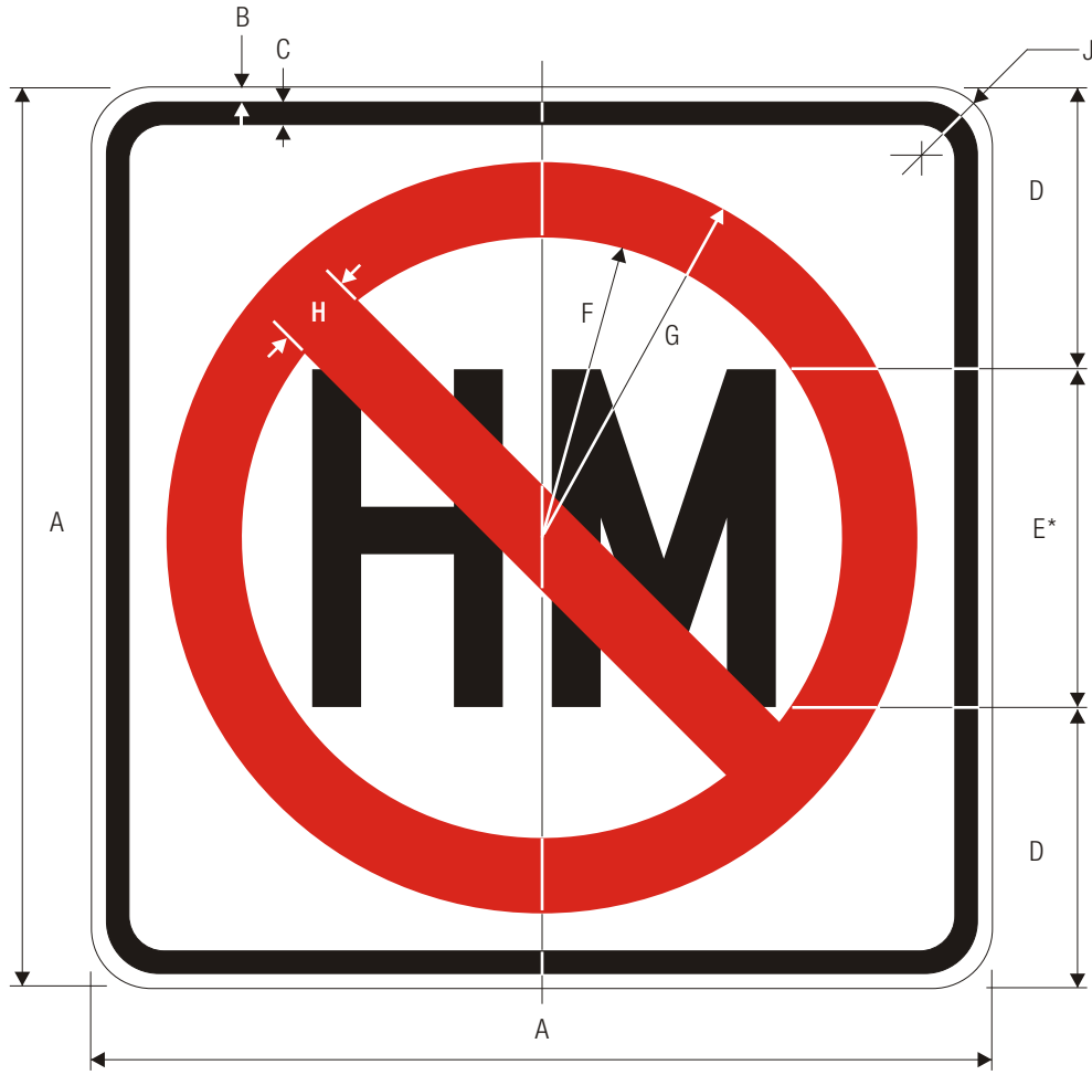
R14-3 HAZARDOUS MATERIAL
