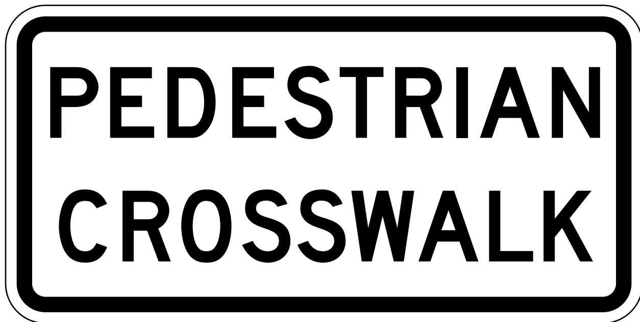
R9-8 Pedestrian Crosswalk
