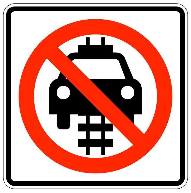
R15-6 (layout per FHWA specifications) No Motor Vehicles On Tracks (symbol)
