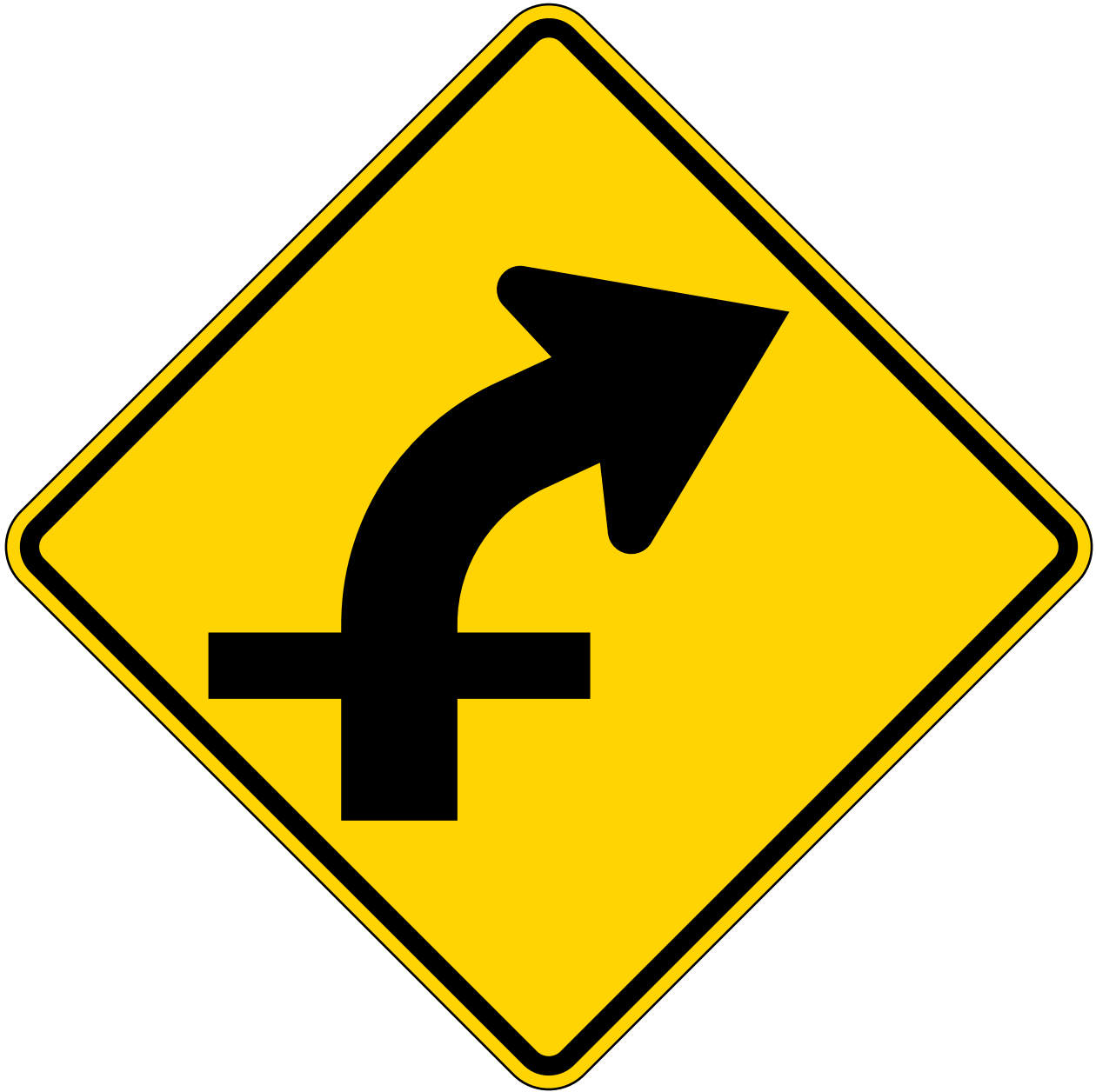
W1-10aR Combination Curve / Cross Road Intersection (Right)
