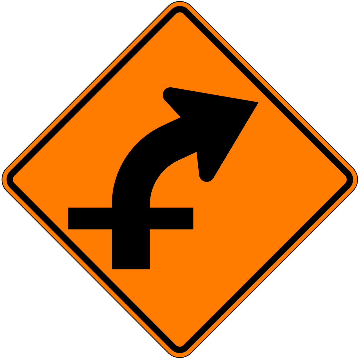
W1-10aR Combination Curve / Cross Road Intersection (Right)
