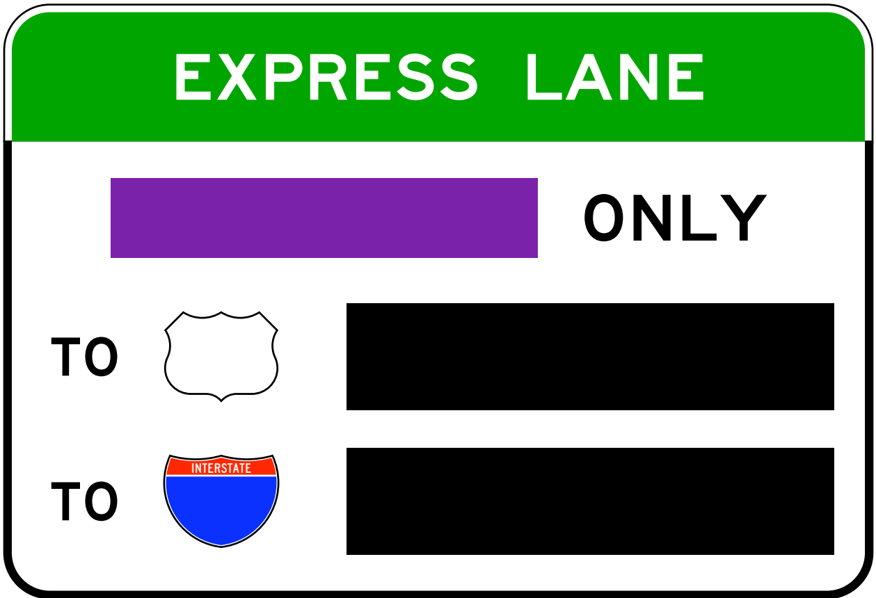
R3-48 Express Lane Toll Rate (Overhead)
