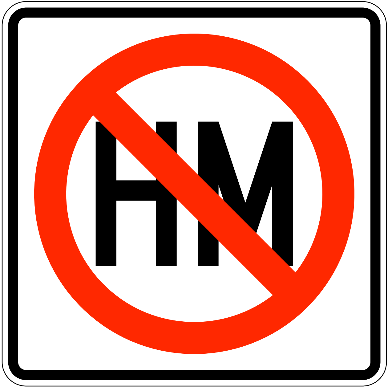
R14-3 Hazardous Material Prohibited
