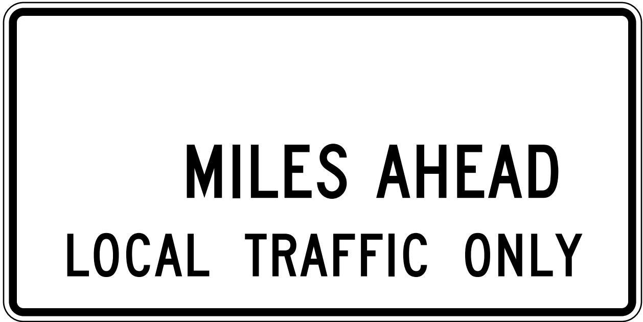
R11-3a Road Closed Ahead Local Traffic Only
