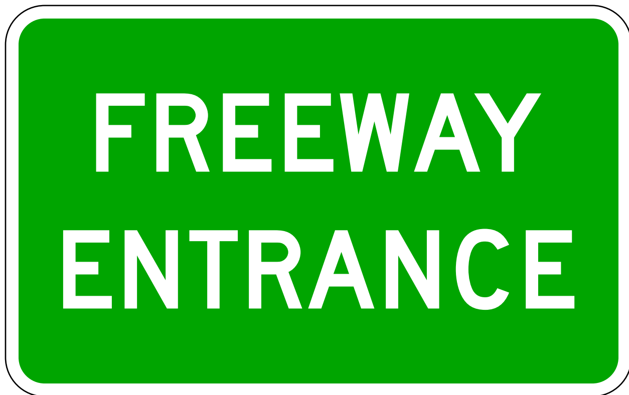
D13-3 Freeway Entrance
