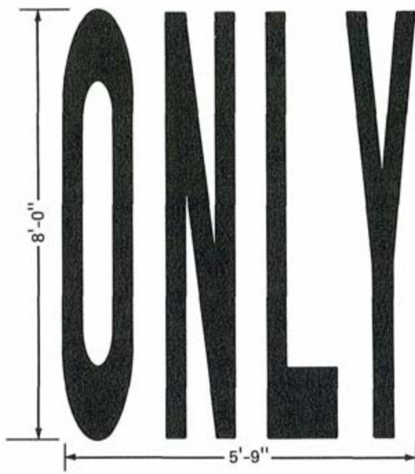
Figure 3-17. Elongated letters for pavement marking.
