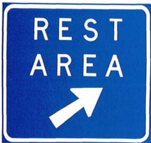
Figure 2-44. Freeway rest area gore sign.
