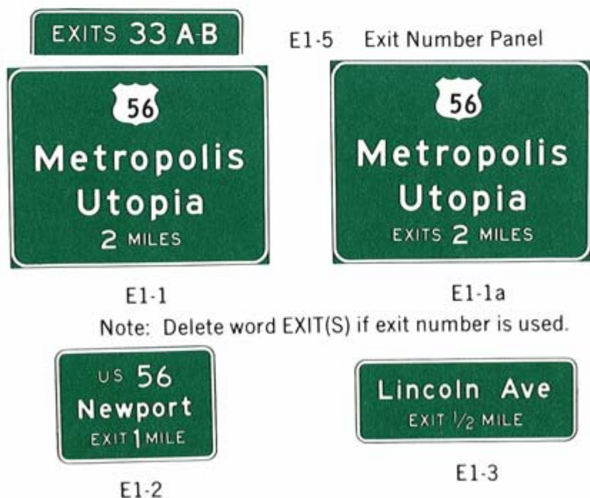
Figure 2-9. Typical interchange advance guide signs.
