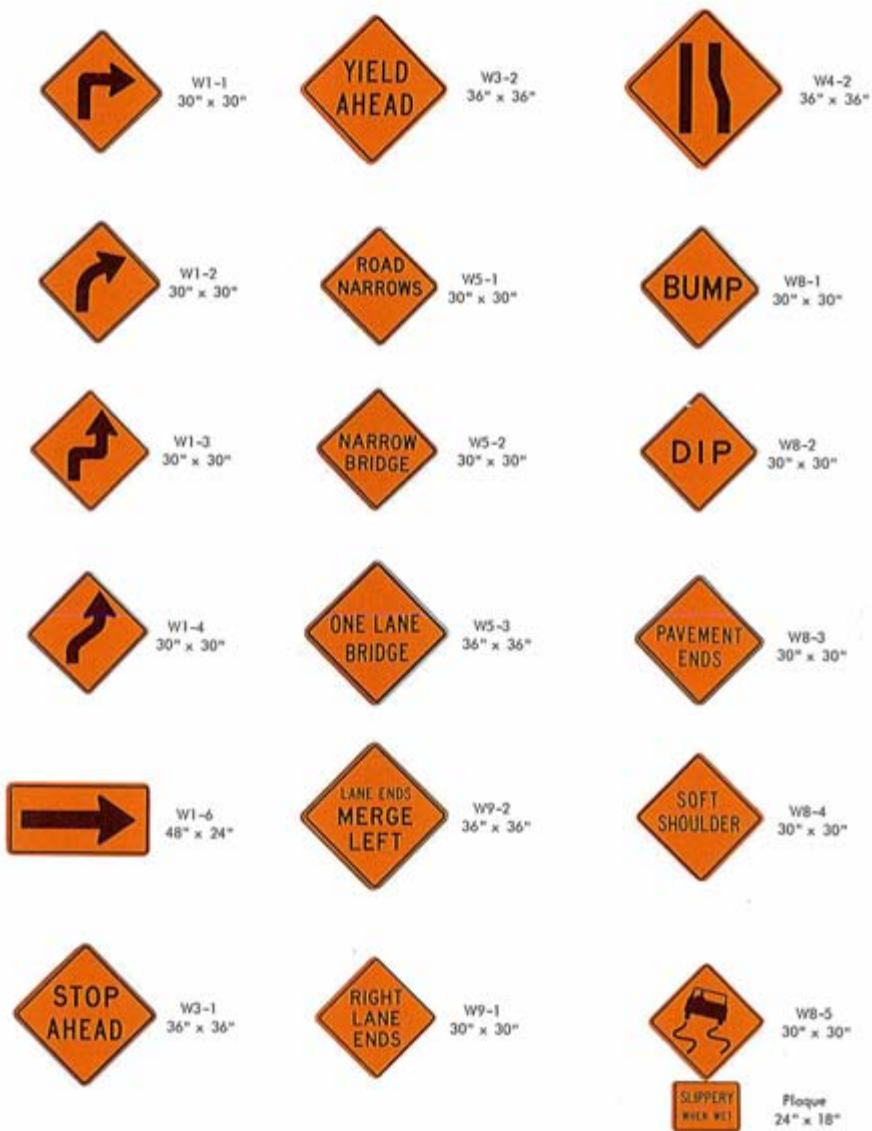
Figure 6-13a. Warning signs used in construction areas.
