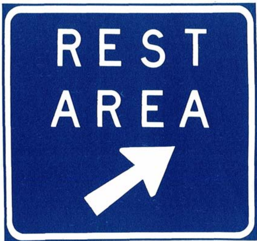
Figure 2-37. Freeway rest area gore sign.
