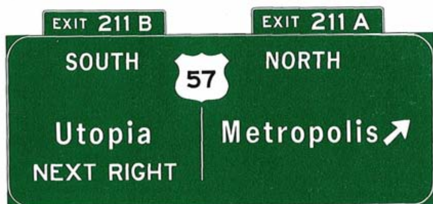
Figure 2-29. Single sign as alternate to two right-hand signs overhead at gore in Figure 2-28.
