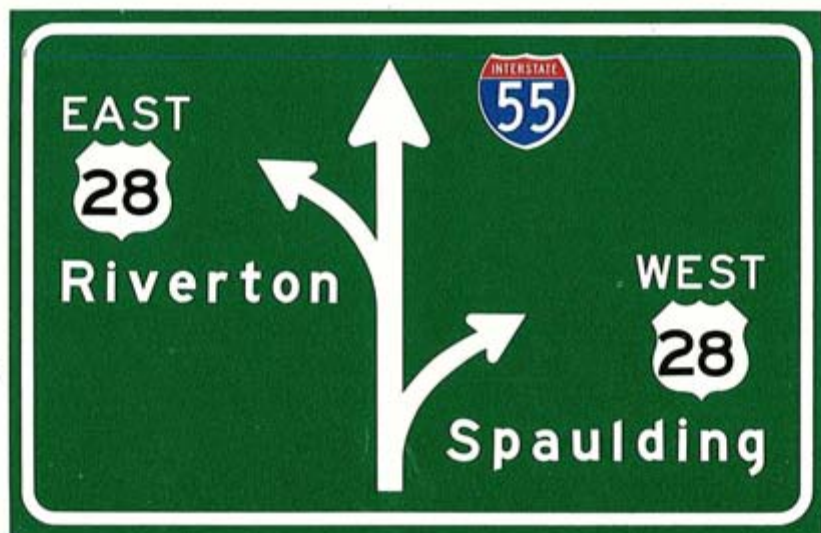
Figure 2-23. Sample diagrammatic sign for directional interchange.
