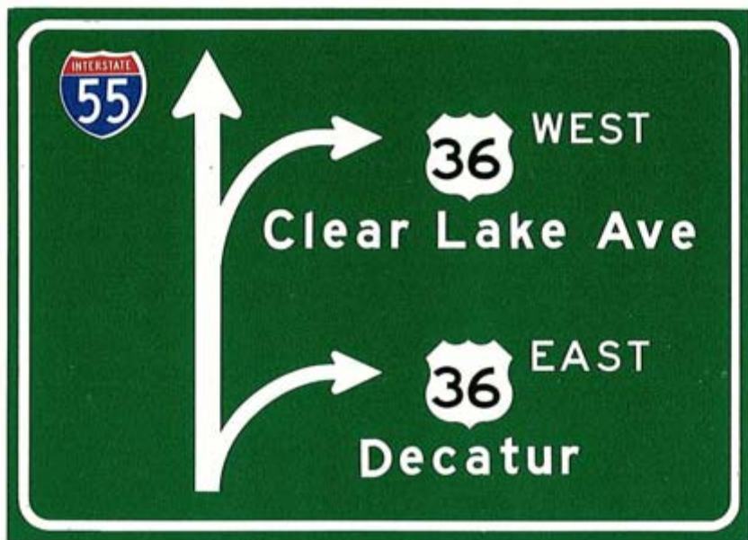
Figure 2-22. Sample diagrammatic sign for cloverleaf interchange.
